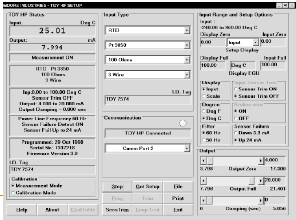
Figure 3. All operating parameters can be set, and then viewed, on a single software screen.
